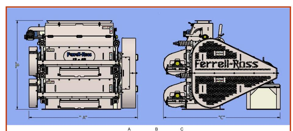
UNIT SHOWN INCLUDES THE OPTIONAL FERRELL-ROSS SCR VARIABLE SPEED ROLL FEEDER
