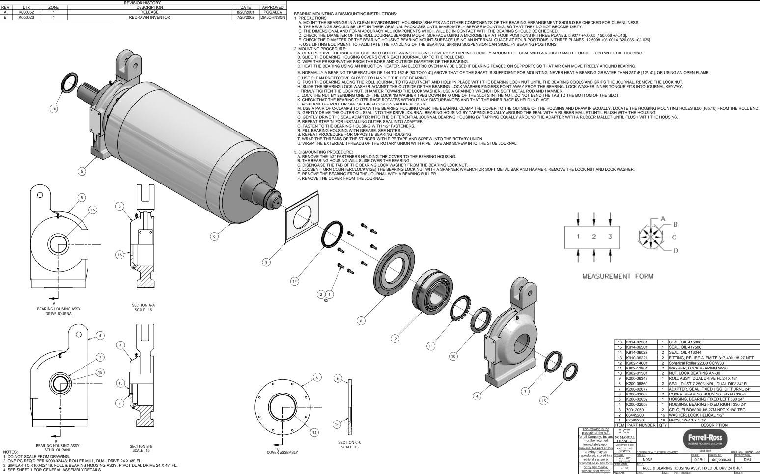
5. FILL BEARING HOUSINGS WITH NLGI №. 2 GRADE LITHIUM BASED GREASE WITH AT LEAST 1000 SSU @ 100 & UNTIL GREASE RELIEFS OPEN, APPROXIMATELY 98 FL OZ (7, 14 OZ TUBES).
